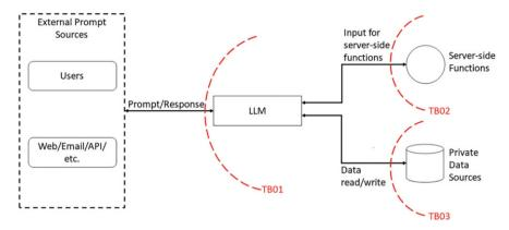
Fig. 27.1 Data flow diagram for attacks on LLM-based applications, based on: [1]
