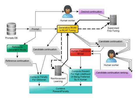
**Fig. 4.1** Iterative refinement of an InstructGPT conversational agent to comply with user expectations, where Step 1 corresponds to first tier CA derivation, while "Step 2 + Step 3" corresponds to the second one. Image courtesy of [3]
